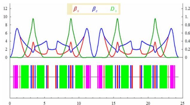
Figure 1: VEPP-2000 lattice (solenoids “on”)
