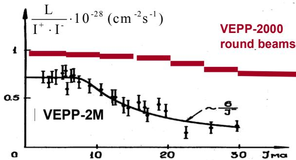
Figure 3: Specific luminosities versus electron current
