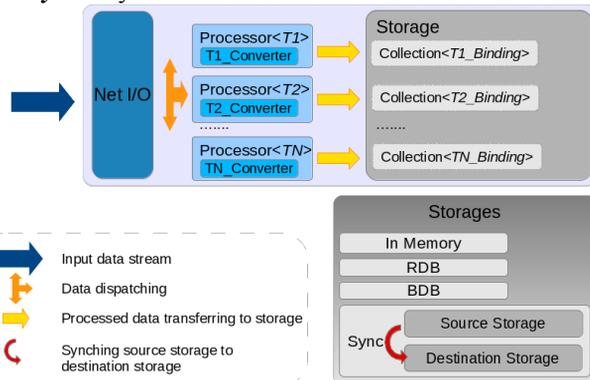
Figure 3: Logging Server structure.
