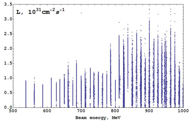
Figure 6: Luminosity measurements in the 2010-2012 runs.
